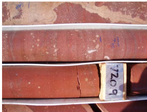
Plate 2: IHAD1 ~720 meters. Post lithification bleaching of earthy infiltration hematite.
