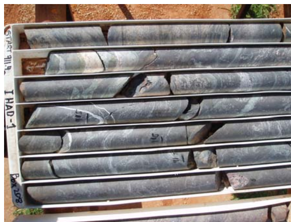
Plate 6: IHAD1 ~915 meters. Brecciated and veined massive magnetite having possible skarn affinities.
