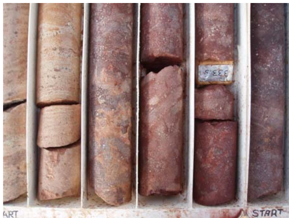
Plate 1: IHAD1 ~333 meters. Intensely brecciated red beds high in the Pandurra sequence passing downward to a long zone of blackened red bed (black seems to represent chlorite and specular hematite in a large plume of alteration)
