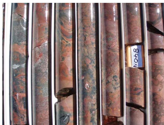
Plate 4: IHAD1 ~841 meters. Jigsaw-brecciated Pandurra Formation sandstone and basalt.
