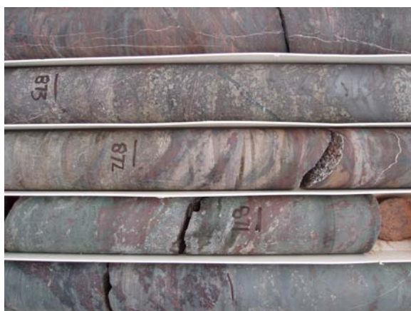
Plate 5: IHAD1 ~872 meters. Foliated chloritic "skarnoid"? showing prominent and stretched hematite clasts rimmed by earthy hematite.
