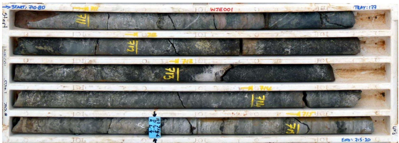
Figure 2: Iron oxide altered basement with localized sulfide commencing two meters below unconformity with cover sequence rocks, WJEDH001.
